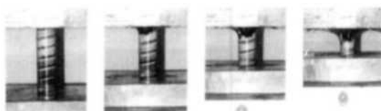
Fig. 4 Collapse process of CF/Epoxy composite tubes with a 0° outer ply orientation angle, SA00N
